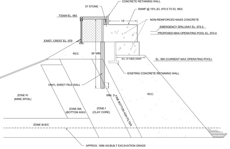
**LB2** SECTION THROUGH EXISTING EMERGENCY SPILLWAY RAMP
