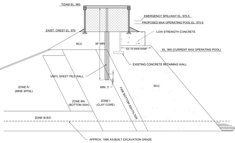
**LB1** SECTION THROUGH EXISTING EMERGENCY SPILLWAY RAMP
