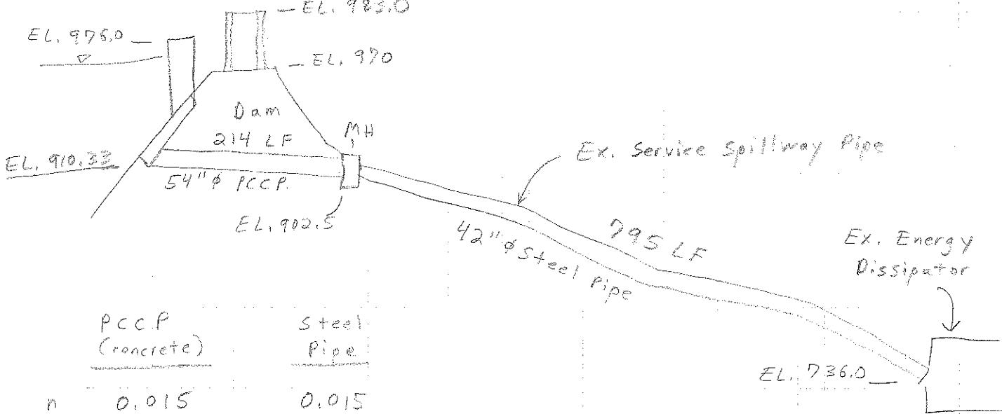
PCCP (concrete)      Steel Pipe
